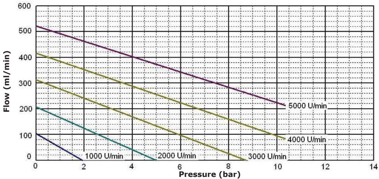
Performance curve based on: medium water, temperature 20°C, viscosity 1 cP, bypass closed
