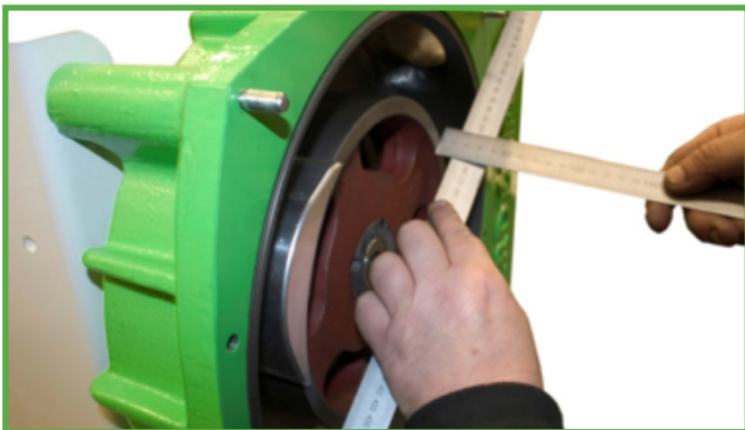
Figure 11 Setting the rotor distance
