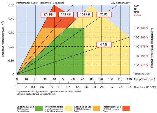
Flows are typical and were measured with water at 68°F with no suction lift or discharge pressure. Actual flows will vary according to suction conditions, discharge pressure and normal component production tolerances.
