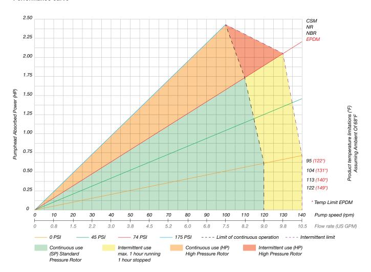
Any application below 15 Hz may require special review. Flows are typical and were measured with water at 70°F with no suction lift or discharge pressure. Actual flows will vary according to suction conditions, discharge pressure and normal component production tolerances.
