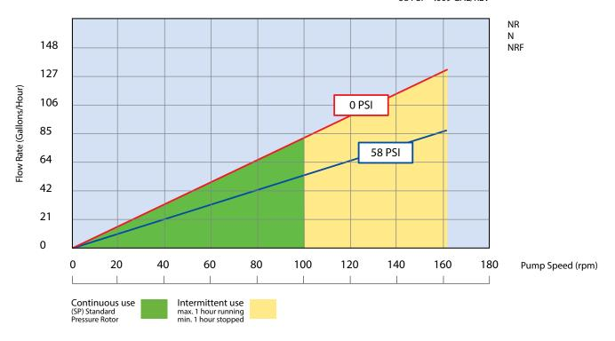
Flows are typical and were measured with water at 68 F with no suction lift or discharge pressure. Actual flows will vary according to suction conditions, discharge pressure and normal component production tolerances.
