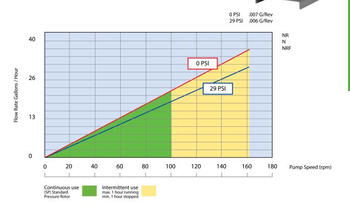
Flows are typical and were measured with water at 68 F with no suction lift or discharge pressure. Actual flows will vary according to suction conditions, discharge pressure and normal component production tolerances.
