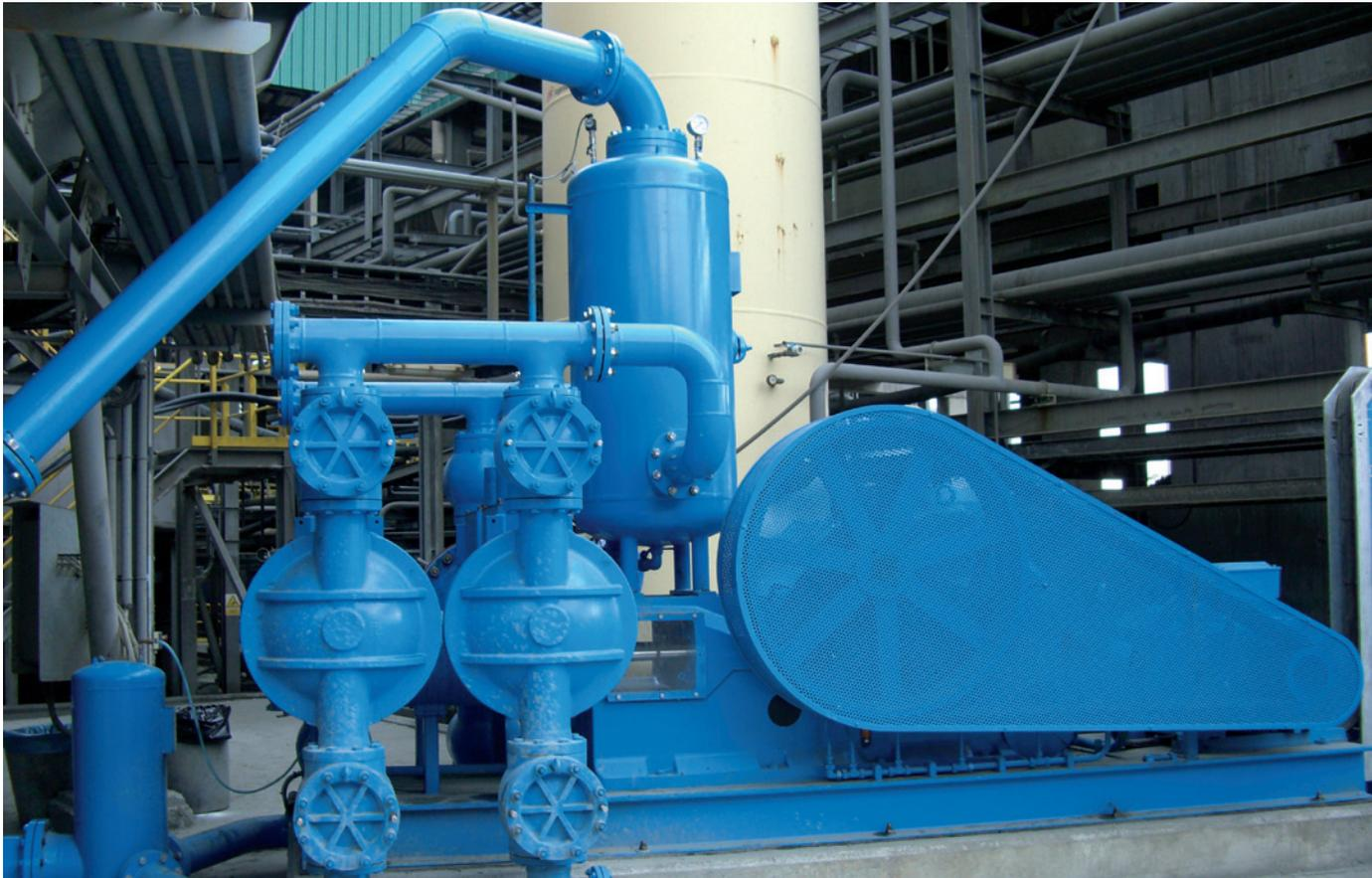
ABEL HMQ for tailings transfer in a copper/nickel mine
