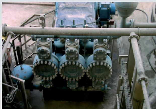
Membrane life times over 8,000 hours are not uncommon and proven on continuous duty
