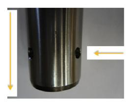
3. Install washer (18) and o-ring (17) on the shaft bolt (16A) (= drilled bolt !)
