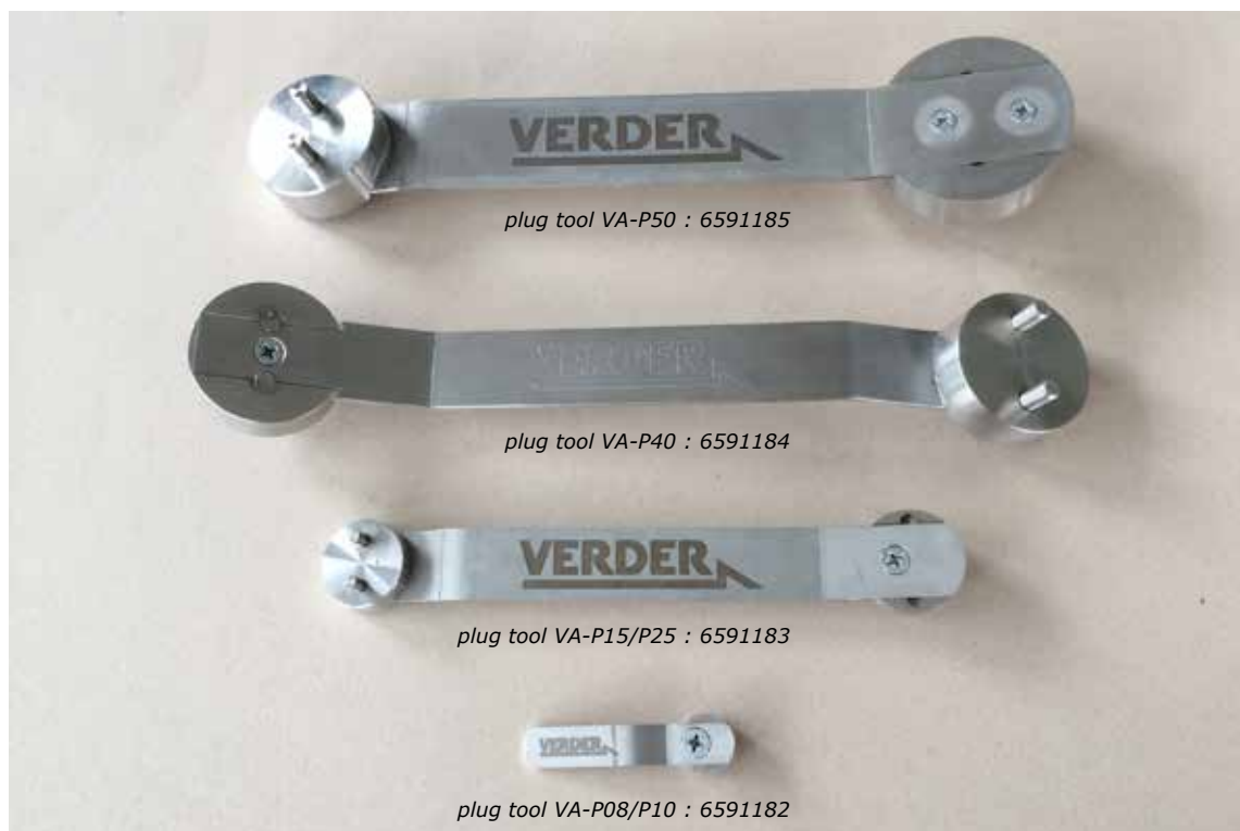
Figure 3b: Set of 4 plug tools
