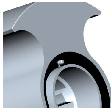
Figure 25 – Align the L cup to the rotor drive pin
