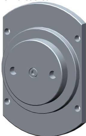
Figure 8 - End cover - thermal jacket
