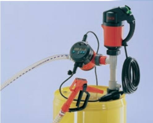
Auto mode: FLUX FMC 100 in conjunction with interface amplifier Type FSV 100 as a presettable batch controller actuating a drum pump
