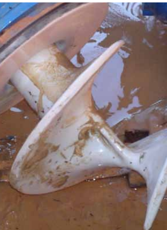
The picture shows the status of the screw after 4 months of action (800 hours).
