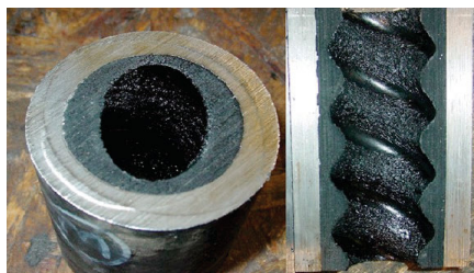
A worn stator; caused by abrasive lime particles. A replacement assembly may cost as much as 25% of the pump + labour costs.
