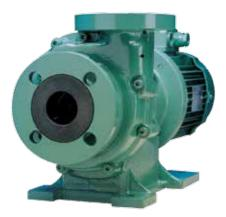
No mechanical seals: No leakage A magnet-driven centrifugal pump offers the best level of protection against leakage. The design itself is leak-free - the pump has permanent magnets with the liquid secured in the pump chamber. The magnetically driven concept requires no mechanical seals subject to abrasive wear between fluid, drive mechanism and the environment.
