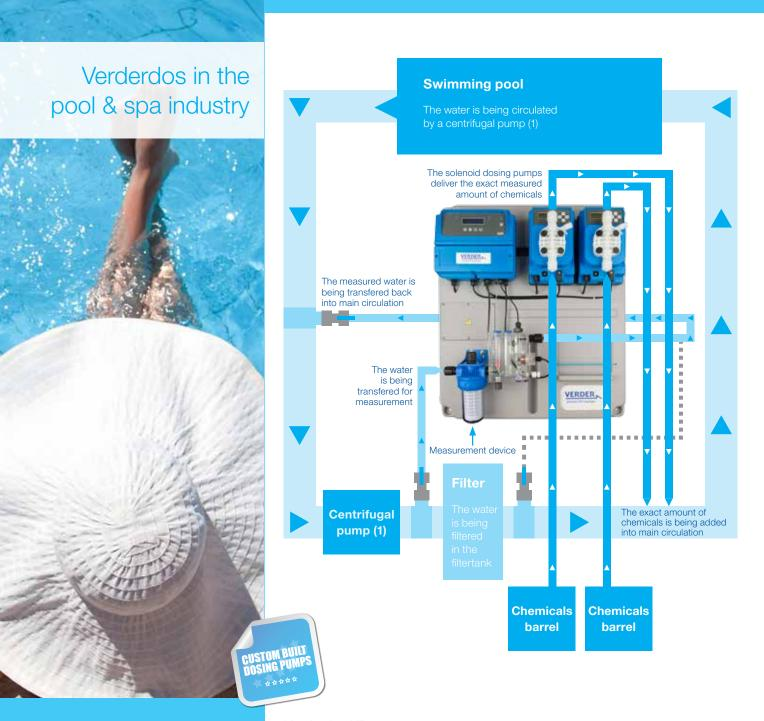
Verderdos and Verderflex VP pumps are ideal pumps for precise dosing in many applications where accuracy is crucial.
