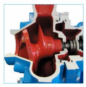
Sectional view of Impeller Housing Assembly
