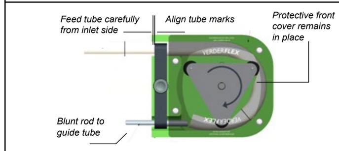
Figure 11 Tube assembly – EV 8000
