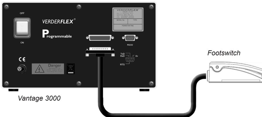
Figure 7 Connecting the footswitch
