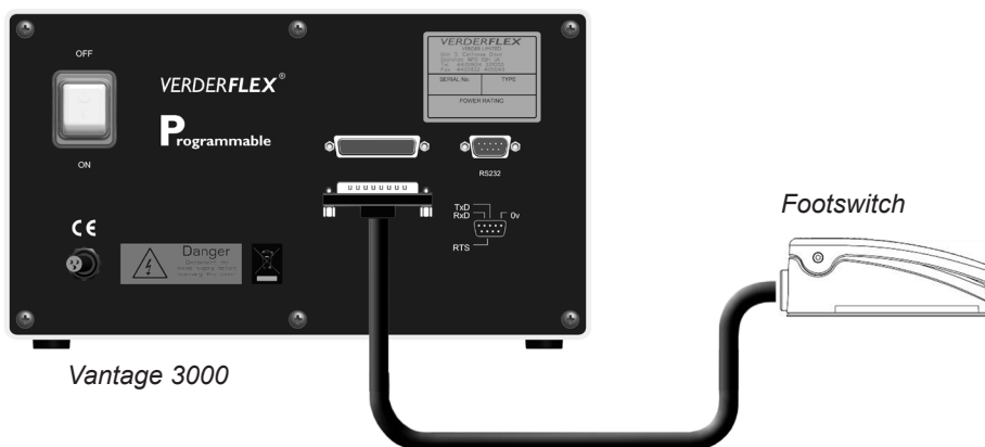
Figure 7 Connecting the Footswitch
