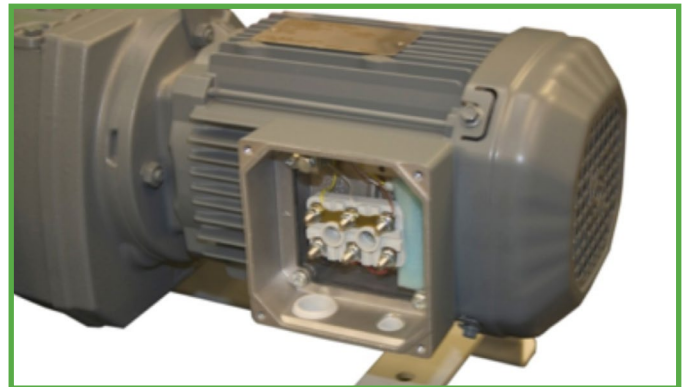
Figure 13 Raccordement du rotor
