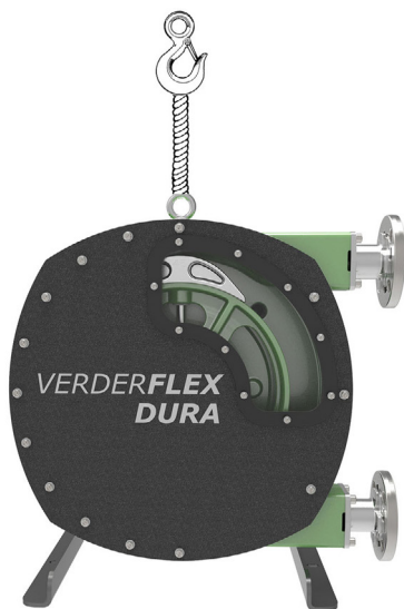
Figure 1 Fastening Lifting Gear to Pump
