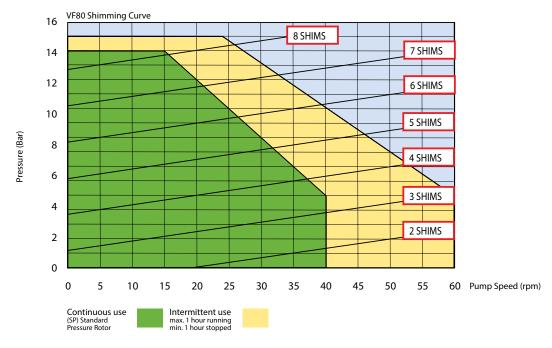
For product temperatures above 65  $^{\circ}$ C and/or viscocity above 2000 mPas use one shim less than shown a contract temperature of the contract temperatures above 65  $^{\circ}$ C and/or viscocity above 2000 mPas use one shim less than shown a contract temperature of the contract temperatures above 65  $^{\circ}$ C and/or viscocity above 2000 mPas use one shim less than shown a contract temperature of the contract temperature of t
