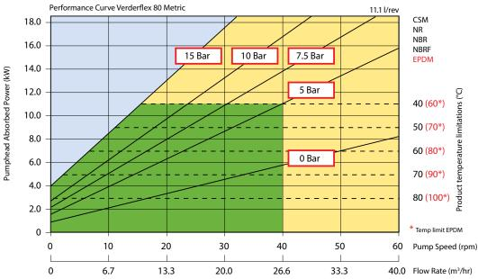
Displacement 11.1 l/revolution, Capacity is speed x 0.67 in m³/hr Minimum starting torque required: 2000 Nm Maximum peak power +9%
