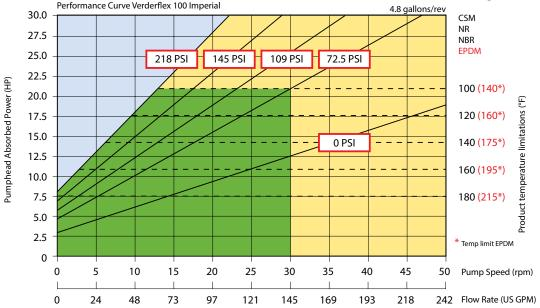
Displacement 4.8 USg/revolution, Capacity is speed x 4.8 in US GPM Minimum starting torque required: 39828 in.Lb Maximum peak power +28%
