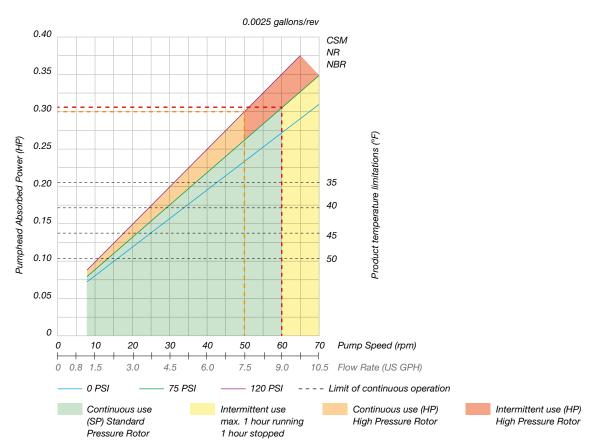
Flows are typical and were measured with water at 68°F with no suction lift or discharge pressure. Actual flows will vary according to suction conditions, discharge pressure and normal component production tolerances.
