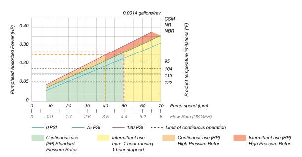
Flows are typical and were measured with water at 68°F with no suction lift or discharge pressure. Actual flows will vary according to suction conditions, discharge pressure and normal component production tolerances.
