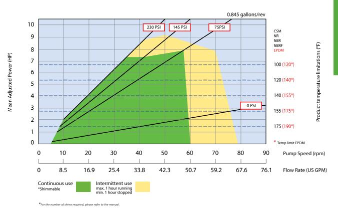
Flows are typical and were measured with water at 65°F with 3 feet suction lift or discharge pressure. Actual flows will vary according to suction conditions, discharge pressure and normal component production tolerances.
