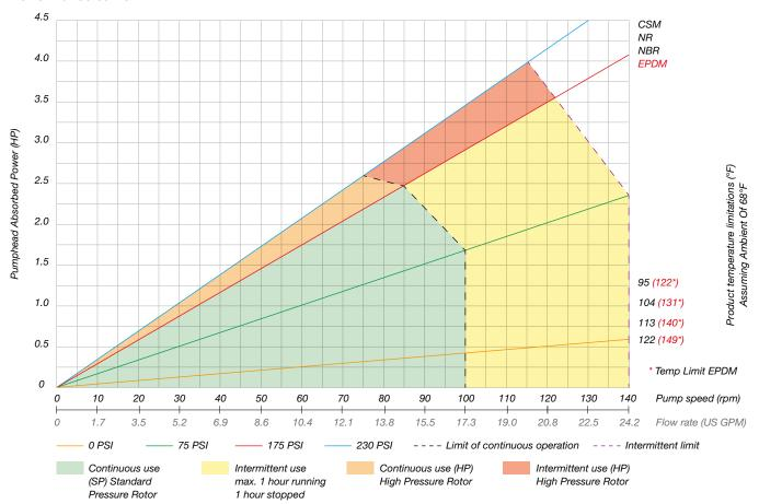
Any application below 15 Hz may require special review. Flows are typical and were measured with water at 70°F with no suction lift or discharge pressure. Actual flows will vary according to suction conditions, discharge pressure and normal component production tolerances.
