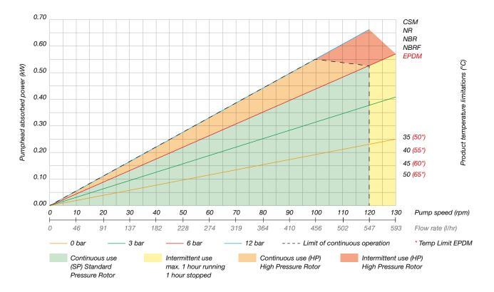
Any application below 15 Hz may require special review. Flows are typical and were measured with water at 20°C with no suction lift or discharge pressure. Actual flows will vary according to suction conditions, discharge pressure and normal component production tolerances.
