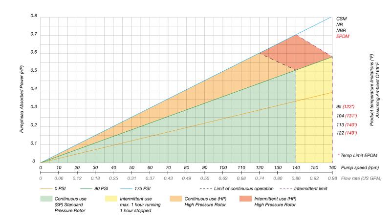
Any application below 15 Hz may require special review. Flows are typical and were measured with water at 70°F with no suction lift or discharge pressure. Actual flows will vary according to suction conditions, discharge pressure and normal component production tolerances.
