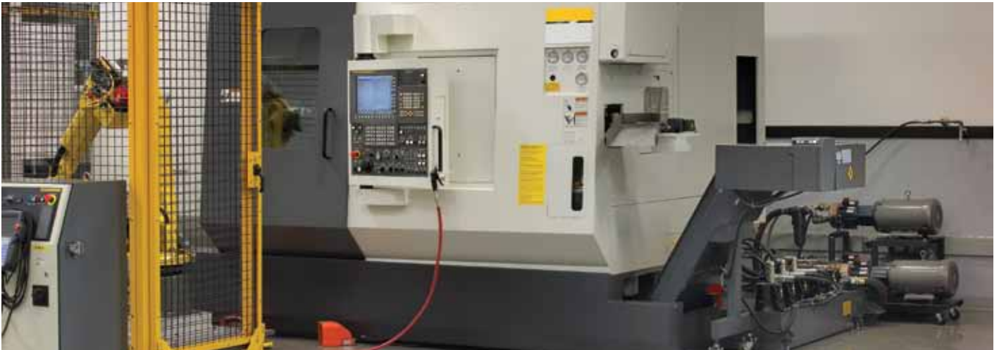
Hydra-Cell pumps deliver high-pressure, controlled flow of machine tool coolant without the need for fine filtration.
