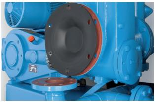
The pre-formed HM membrane is not subjected to any elongation during the entire stroke
