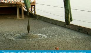
Thickened, digested sewage sludge, 7% solids concentration.
