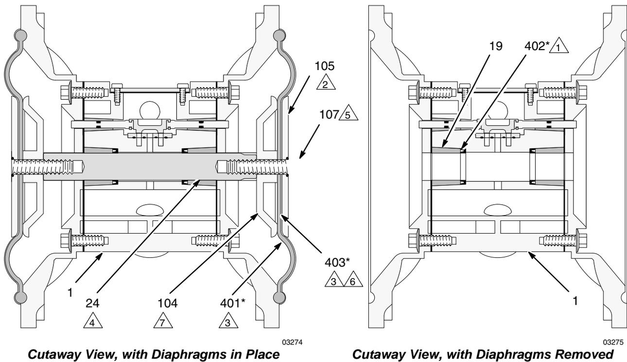
Cutaway View, with Diaphragms in Place
