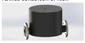
The flange connection is an optional type of PD-S pulsation dampener connection to the installation / pump. Consists of two flange sleeves and two DIN flanges. Flange connections have been prepared in the range of PD-S25 to PD-S80
