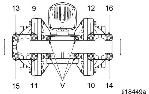
**FIG. 9. Torque sequence**
