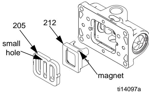
**FIG. 5. Air valve cup and plate installation**
