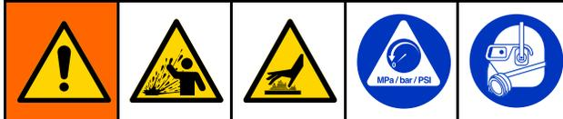
This equipment stays pressurized until pressure is manually relieved. To help prevent serious injury from pressurized fluid, such as splashing fluid, follow the Pressure Relief Procedure when you stop dispensing and before cleaning, checking, or servicing the equipment.
