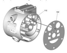
5. Align the air cover (103) so the pilot pin (112) fits in the middle hole (M) of the three small holes near the center of the cover.
