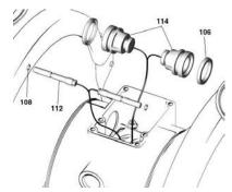
Install u-cups (106) on each actuator piston (114), so the lips of the packings face the *narrow* end of the pistons. 5. Grease the lower face of the pilot block (116) and install so its tabs snap into the grooves on the ends of the pilot pins (112).
